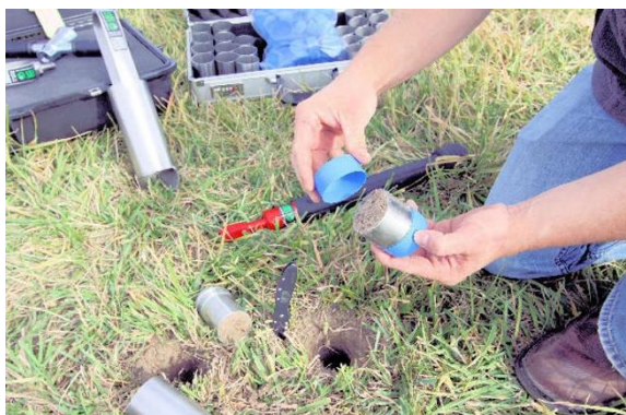
Fig.6.2 Recoltarea probelor de sol cu cilindrii metalici ( https://certifiedmtp.com/bulk-density-soil-sampling-kit-with-hammer-head-handle-5-8in/#&gid=1&pid=4 )
